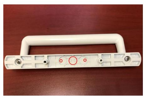
2. Mark the 5/8" hole center using the hole center punch. Make sure the handle is secured in place for drilling via a vise etc. then use the center drill to drill the pilot hole for the 5/8" hole. Progressively use larger drill bits until the 5/8" hole size is achieved. Use the
